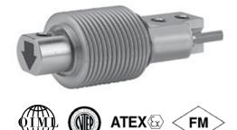
The low profile, high accuracy and sealing makes this load cell highly suitable for applications such as low profile platforms, weighing and packing machines, conversion of mechanical scales and variety of other applications where sealed cells are required. For hazardous environments this load cell is available with EEx ia IIC T6 level of approval as an option.
